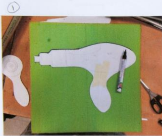
1 3D ANGLE ORTHOGONAL DRAWINGS ARE TRANSFERRED ONTO THE FOAM BLOCK.
