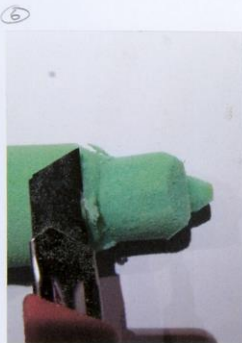
6 A RAZOR BLADE WAS USED TO BLOCK OUT AND CLEAN UP FORM.
