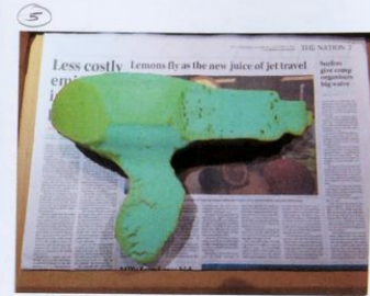
5 THE CUT FOAM WAS PULLED FROM THE MAIN BLOCK.
