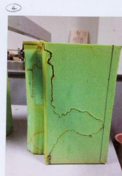
5 THE CUT FOAM WAS PULLED FROM THE MAIN BLOCK.
